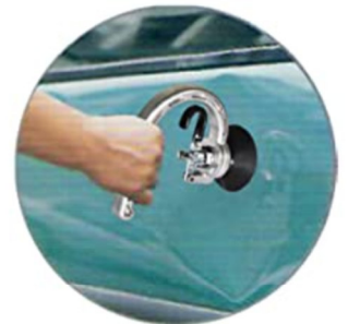
Use as manual auto sheet metal dent puller, PDR work won't damage the paint. The dent dimension must be completely smaller than the pad or should be Larger than the suction pad (over 5.9 inch (150 mm) of dia.) and the surface must be flat to be sucked by the pad easily.
