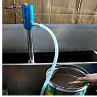
Pumping CNC Oil Out Of A Opening Container
